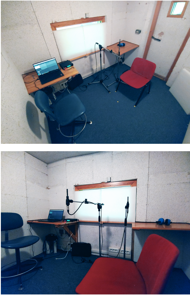
Fig. 1: The acoustically-treated chamber where the speeches were recorded along with the measurement setup. The participant was seated on the red chair, while the experimenter was seated on the blue one.
