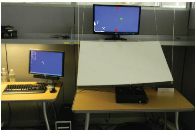
Fig. 6. Error-related auditory feedback: experimental setup at UCI with a 2-DoF force-feedback joystick.
