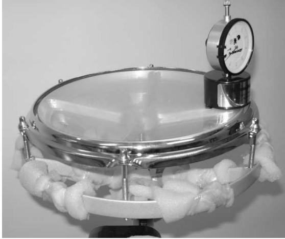
Figure 2: Recording setup: the membrane is tuned with a precision tuner, and the support is damped with foam.
