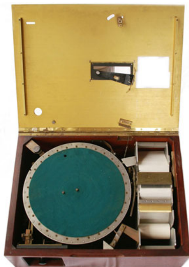
Fig. 1.1 Skinner's teaching machine: paper disks containing the educational programs were inserted into the wooden box and the text appeared in the window on the cover. Lifting a lever in the front allowed the student to check the response and advance to the next frame. Picture from Wikimedia Commons ( https://upload.wikimedia.org/wikipedia/commons/2/2d/Skinner_teaching_machine_08.jpg )
