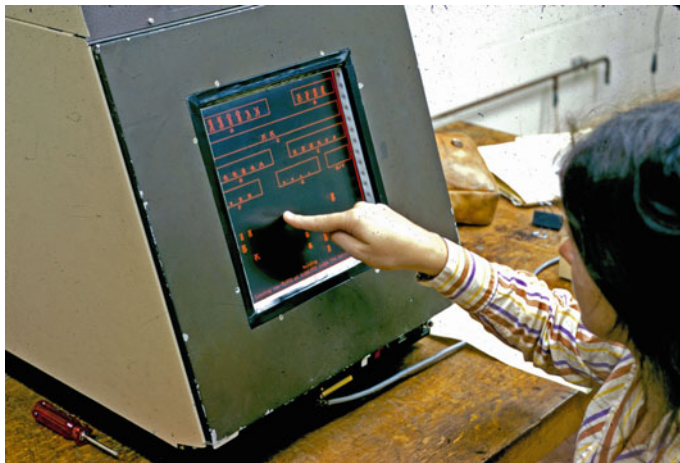
Fig. 1.3 Interactivity with the first touchscreen implemented for the PLATO IV system. Image with permission from Paul J. Tenczar, University of Illinois
