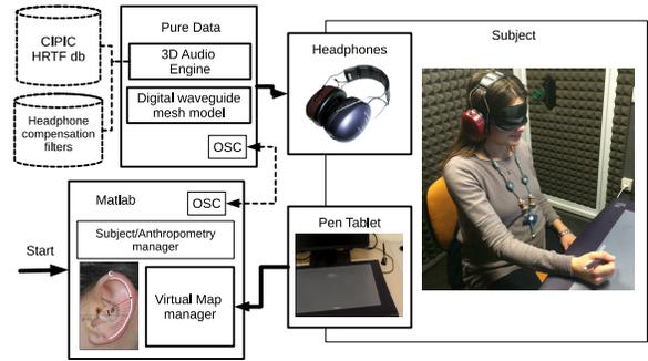
Figure 1: A schematic view of the system architecture.
