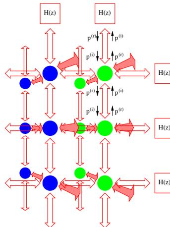
Figure 2: Particular of the 3D DWM: scattering junctions and boundary filters.
