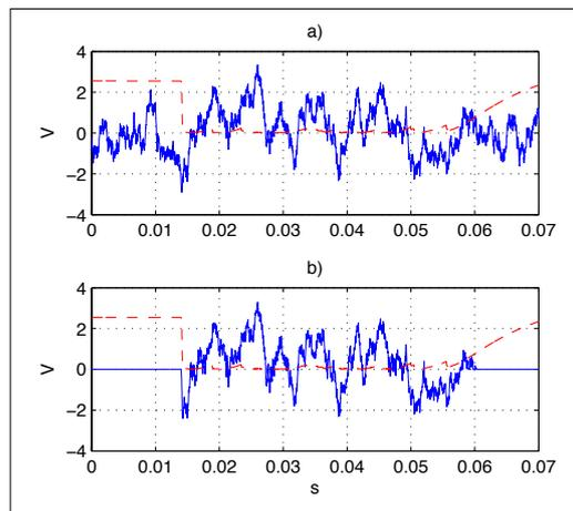
**Figure 6.** Spice simulation of the circuit excited with a stochastic signal. a) input signal (blue solid line) and the voltage  $V_p$  (red dotted line); b) output signal (blue solid line) and the voltage  $V_p$  (red dotted line). The selector is turned on  $C_1 = 0.01\mu F$ .
